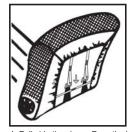
Pull side ties down. Pass the long tie under the seat (or) behind the seat floor mountings and simply attach by pressing together.
