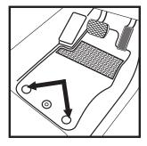
STEP 1: Lay floor mat in place and position outside holes in mat to accommodate existing vehicle lock downs.
