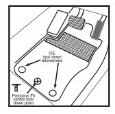
STEP 4: Re-position the floor mat as per step 1. Use lock down fastener to secure mat via centre lock down point.
