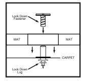
STEP 3: Remove mat and screw in lock down lug directly into carpet/floor lining.
